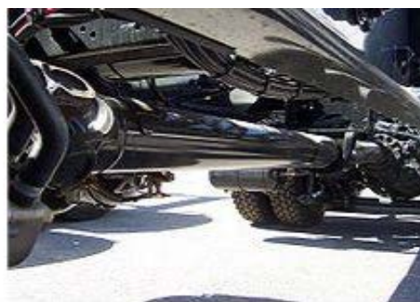
Fig:2.1 A truck double propeller shaft
