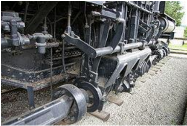
Fig:2.3 The rear drive shaft, crankshaft and front drive shaft of a Shay locomotive
