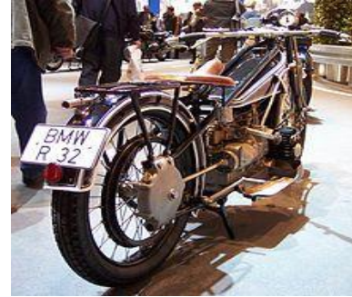
Fig:2.2 The exposed drive shaft on BMW's first motorcycle, the R32
