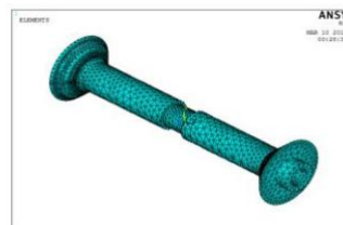
Fig:1 Boundary condition on driven shaft
